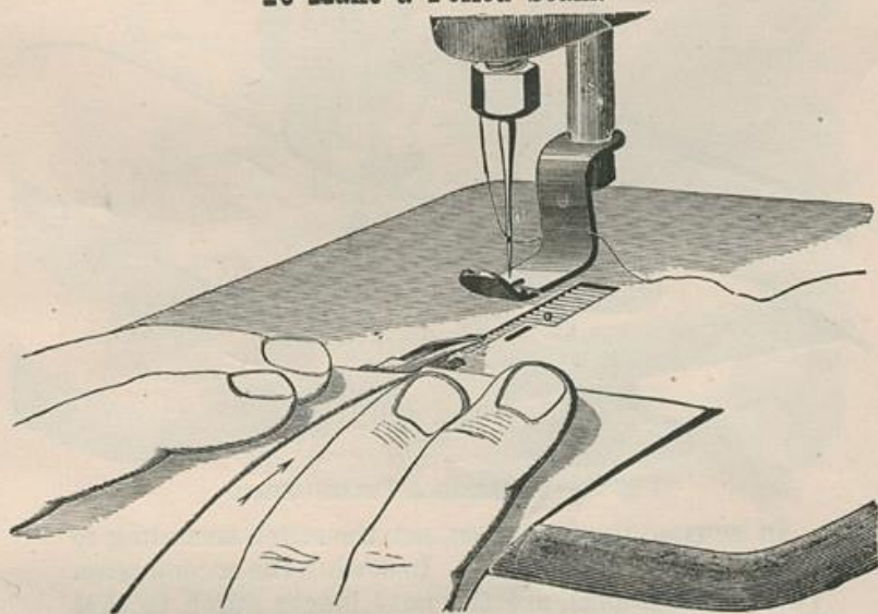
Fig. 22.—INSERTING SEAM TO BE FELLED.
