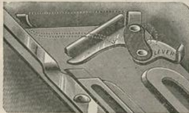
Fig. 2.—Showing Guide adjusted for Narrow Tucks.
