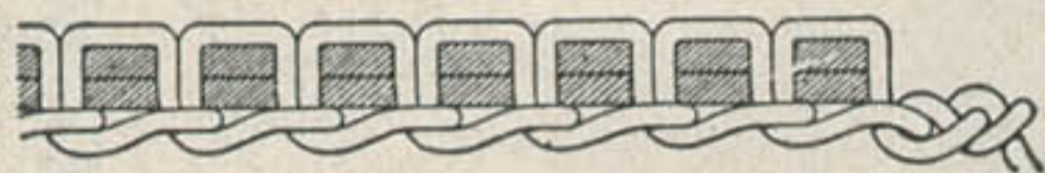
FIG. 4. STITCHING FASTENED AT THE END OF A SEAM
